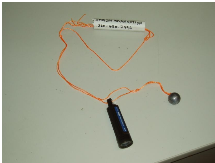
Figure 3: assembled sensor package prior to deployment. A fishing bobber was added to enhance visibility in eelgrass beds.
