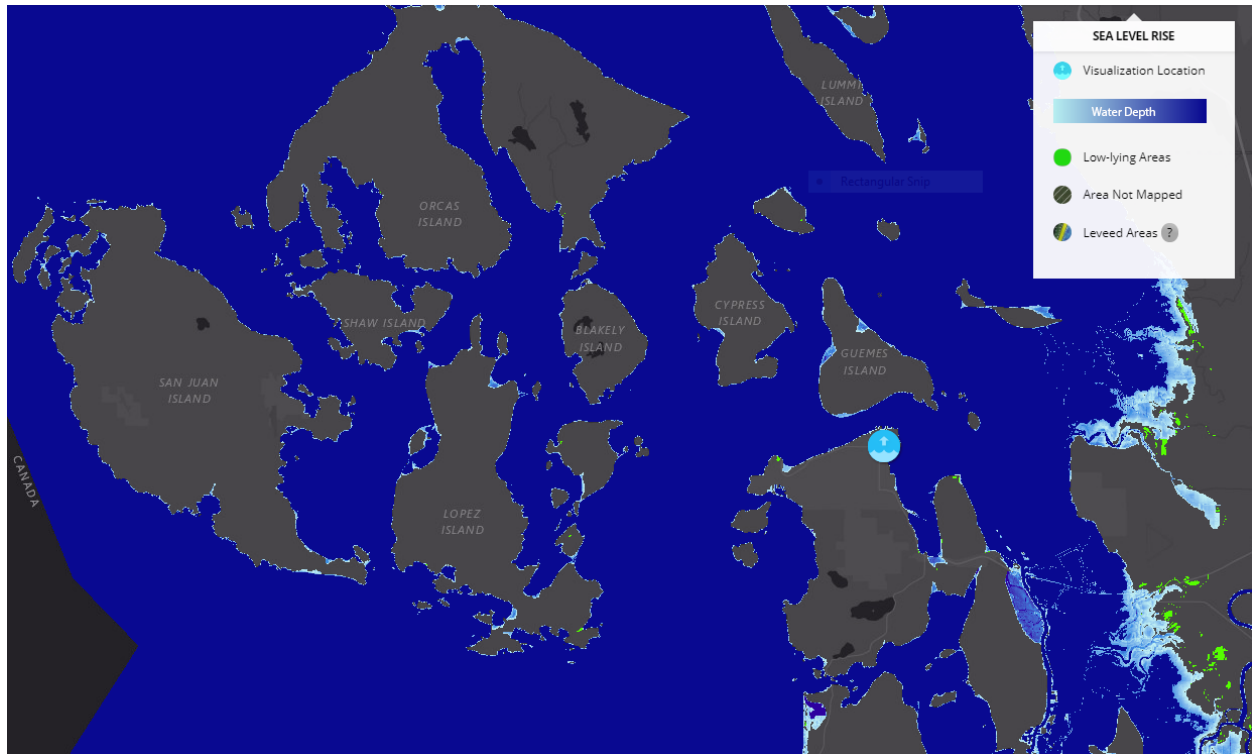
Figure 16: Visualization showing estimate of areas potentially inundated by 5-foot increase in sea levels (shown in blue, with darker blue indicating greater depth of water). Inundation is shown as it would appear during MHHW—the average of the higher high-water height of each tidal day observed over the National Tidal Datum Epoch. The data in the maps do not consider natural processes such as erosion, subsidence, or future construction. Figure Source: NOAA Sea Level Rise Viewer.
