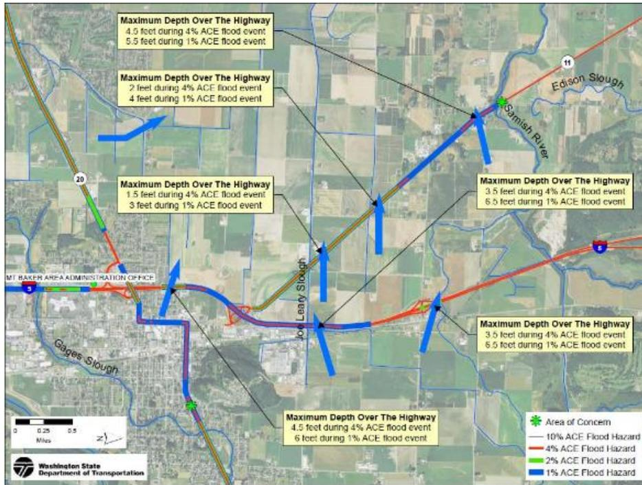
Figure 10 Northern section of WSDOT flood hazard study area showing I-5, SR 20, and SR 11. Arrows indicate flow of water. Note: top of map is west. (WSDOT, 2015).
