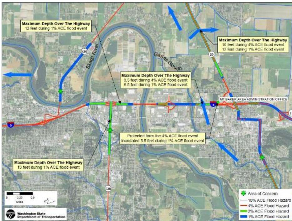
Figure 11 Northern section of WSDOT flood hazard study area just south of previous figure, showing I-5, SR 20, and SR 538. Arrows indicate flow of water. Note: top of map is west. (WSDOT, 2015).
