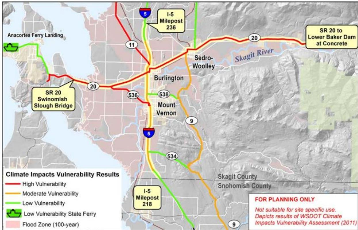
Figure 7 Map showing stretches of state and federal highways that are vulnerable to climate change assuming 2 ft of sea level rise based on GIS flood analysis. (WSDOT, 2011).
