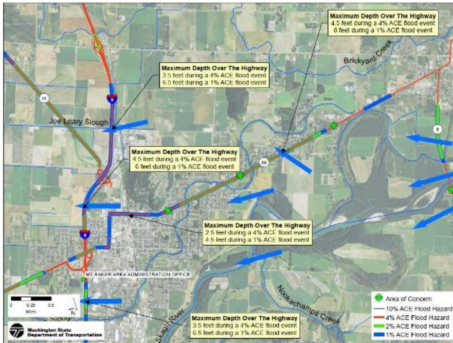
Figure 14 East section of WSDOT flood hazard study area, east of Burlington, including SR 538, SR 9, SR 20, and I-5. Note: Arrows indicate flow of water. (WSDOT, 2015).
