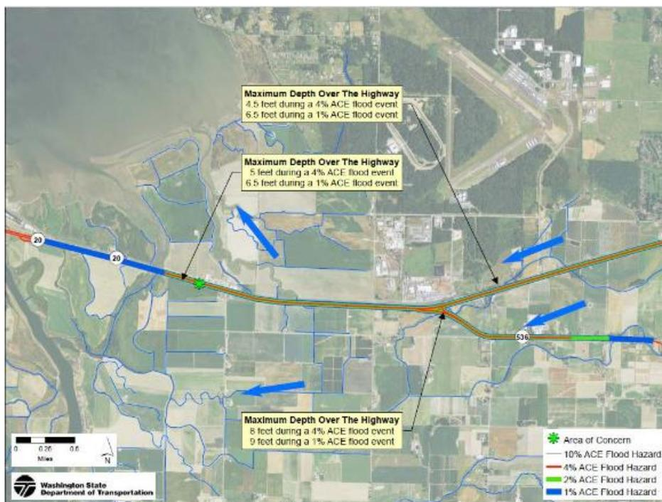
Figure 13 West section of WSDOT flood hazard study area, west of I-5, showing SR 20 and SR 536. Note: Arrows indicate flow of water. (WSDOT, 2015).
