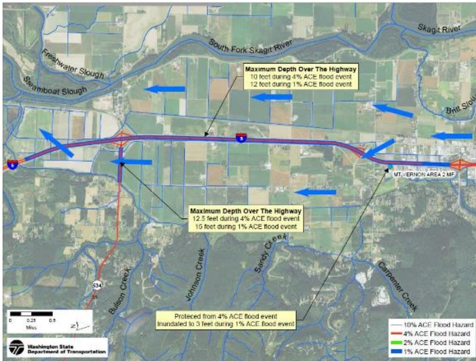
Figure 12 Southern section of WSDOT flood hazard study area, south of Mount Vernon, showing I-5 and SR 534. Arrows indicate flow of water. Note: top of map is west. (WSDOT, 2015).
