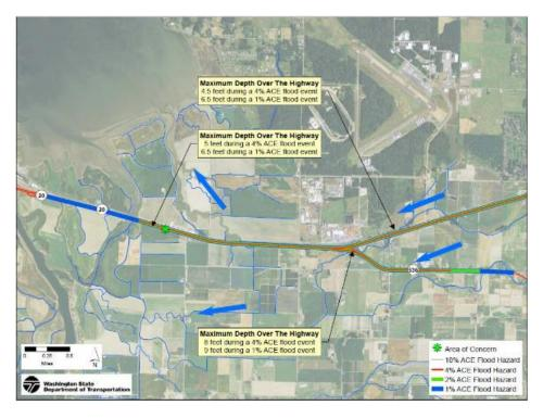
Figure 13 West section of WSDOT flood hazard study area, west of I-5, showing SR 20 and SR 536. Note: Arrows indicate flow of water. (WSDOT, 2015).
