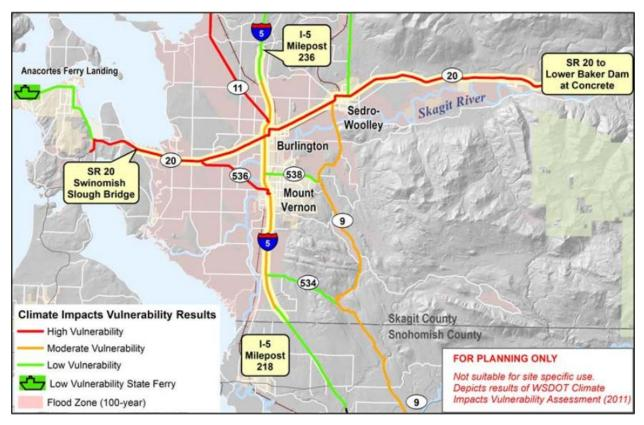
Figure 7 Map showing stretches of state and federal highways that are vulnerable to climate change assuming 2 ft of sea level rise based on GIS flood analysis. (WSDOT, 2011).
