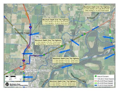
Figure 14 East section of WSDOT flood hazard study area, east of Burlington, including SR 538, SR 9, SR 20, and I-5. Note: Arrows indicate flow of water. (WSDOT, 2015).
