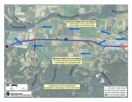
Figure 12 Southern section of WSDOT flood hazard study area, south of Mount Vernon, showing I-5 and SR 534. Arrows indicate flow of water. Note: top of map is west. (WSDOT, 2015).
