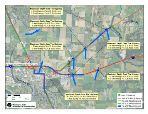
Figure 10 Northern section of WSDOT flood hazard study area showing I-5, SR 20, and SR 11. Arrows indicate flow of water. Note: top of map is west. (WSDOT, 2015).
