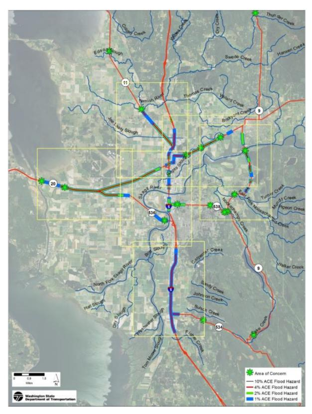
Figure 9 WSDOT study area with flood hazard locations for 1%, 2%, 4% and 10% ACE floods. (WSDOT, 2015).
