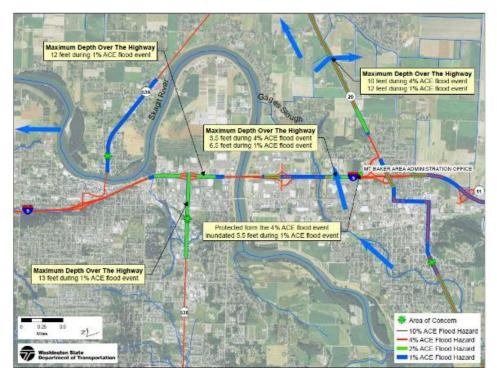
Figure 11 Northern section of WSDOT flood hazard study area just south of previous figure, showing I-5, SR 20, and SR 538. Arrows indicate flow of water. Note: top of map is west. (WSDOT, 2015).
