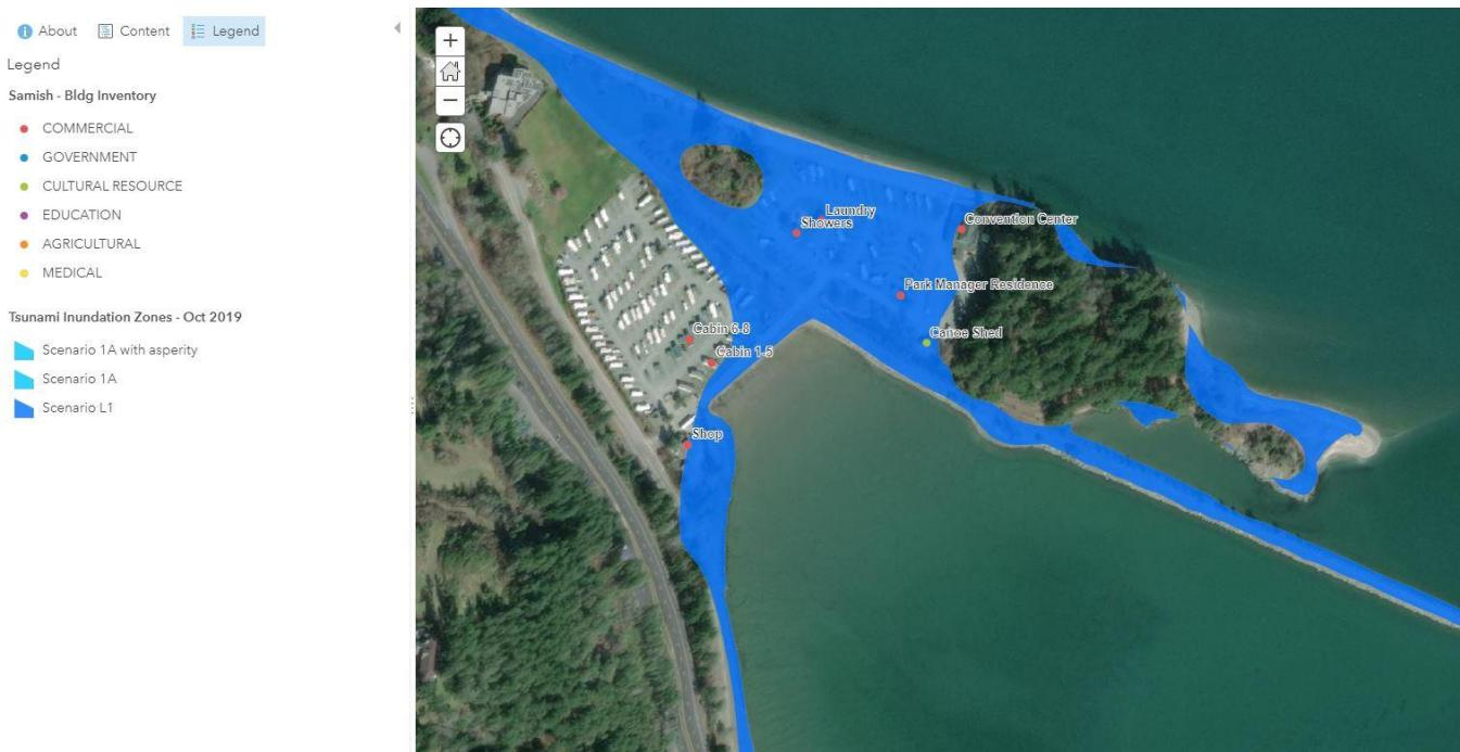
Figure 11-10 Aerial Imagery of Tsunami Inundation Zones Building Impact
