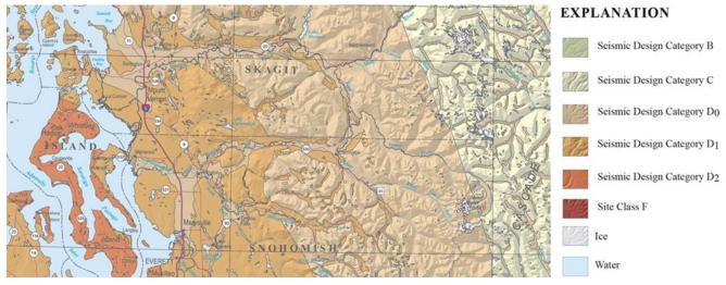
Figure 7-3 Seismic Design Codes
